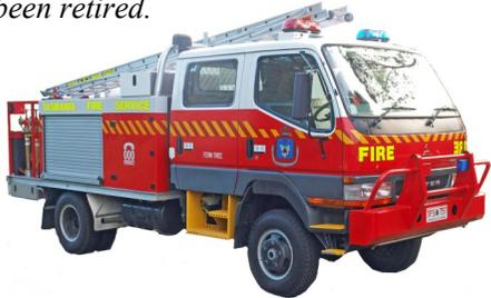
In its place we have been allocated a medium tanker/pumper appliance. Built on a 2005 Mitsubishi Canter twin cab 4x4 chassis, before coming on strength, our new appliance was modified and upgraded to meet the specific needs of our brigade and the broad range rinks in our district.
